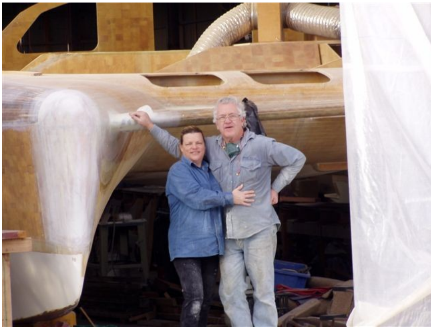
The proud builders, Paul + Wendy. Paul's hand is on that strongpoint for the bridle and striker.
